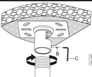
Insert and tighten one set screw to secure it.
